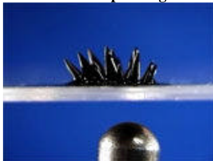
Figure 1: A ferrofluid responding to a cow magnet
